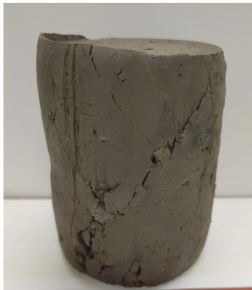
Unconfined Compression Test/UU Triaxial Test ASTM D2850-03a - Unconsolidated-Undrained Test N6225271 Project Name: Medina Lake Trail B-8 Depth: 21.0 - 23.0 Sar
